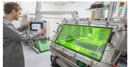
Additive manufacturing system using LDED technology
