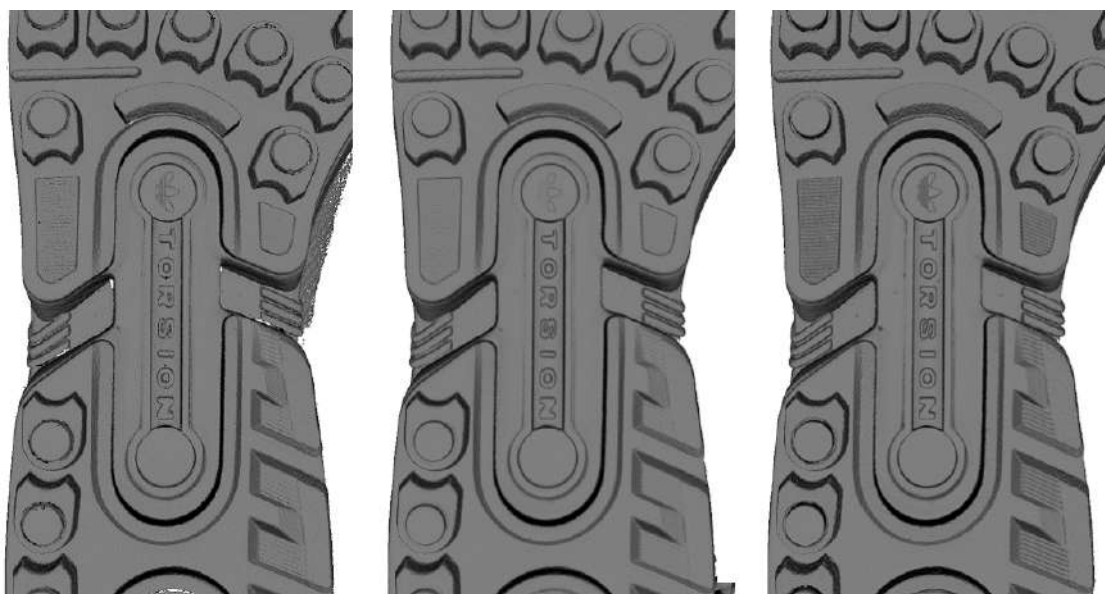
Figure 93: Models of a shoe sole obtained using various algorithms: Fast fusion (left), Smooth fusion (middle) and Sharp fusion (right).
