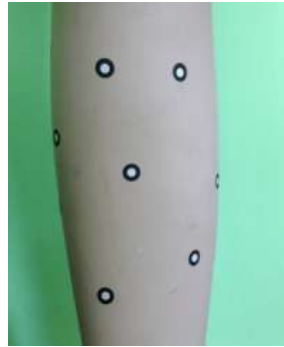
Figure 46: Non-coded targets placed on an object.
