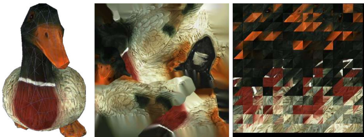
Figure 111: Texture mapping methods: mesh with texture applied (left), texture-atlas sample (middle) and triangle-map sample (right). The latter covers only a portion of the mesh surface (the rest two images not shown).
