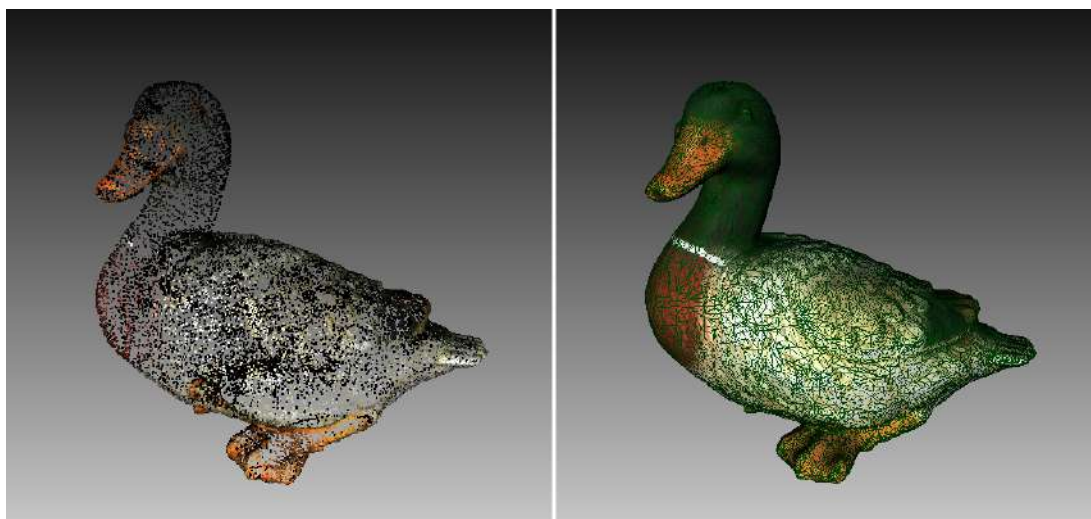
Figure 62: Examples of model using different rendering modes. Point model on left and wire over solid on right.
