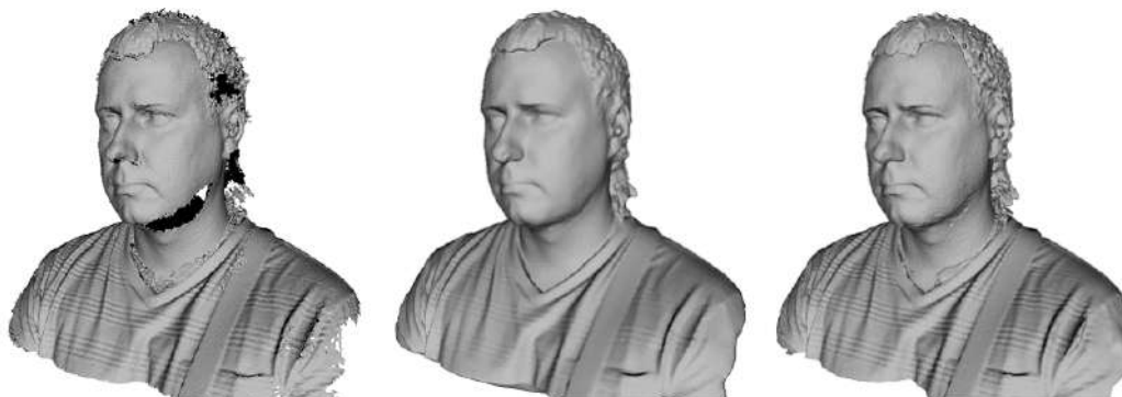
Figure 92: Models of a human subject obtained using various algorithms: Fast fusion (left), Smooth fusion (middle) and Sharp fusion (right).
