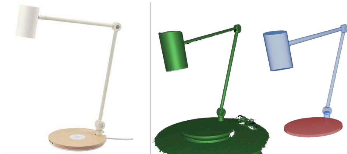
Figure 124: From left to right: original object, scanned model, a set of constructed primitives.
